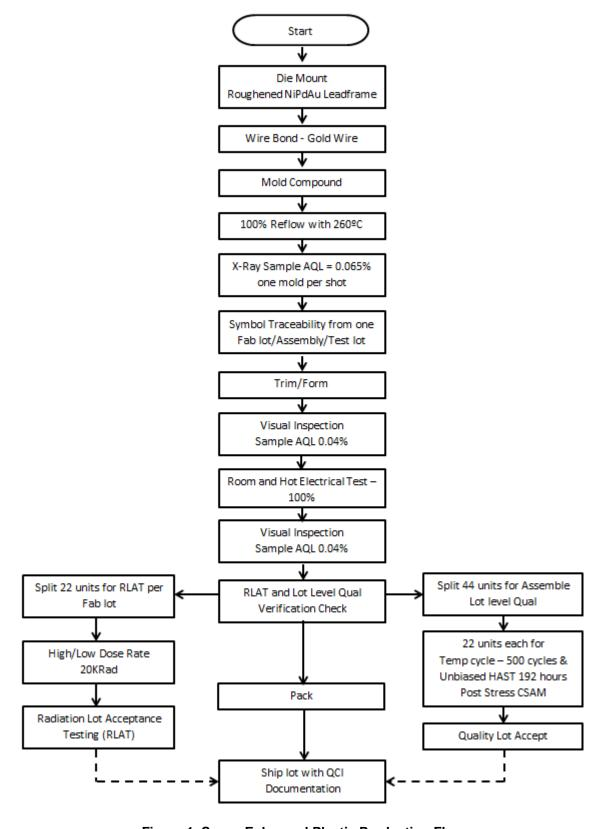
Figure 1. Space Enhanced Plastic Production Flow
