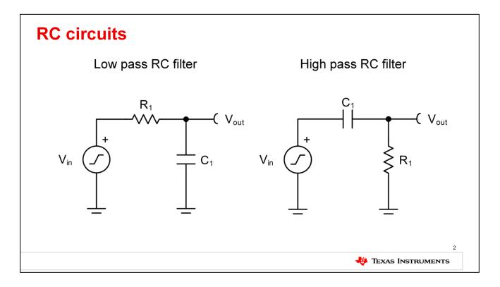
RC circuits are composed of resistive and capacitive elements. They can be formed in one of the two ways shown here. RC circuits can be both intentionally designed and occur parasitically. Because they are so commonly seen with op amps, understanding their function is important for analog designers. In this presentation, we will observe both the transient and AC response of RC circuits.
