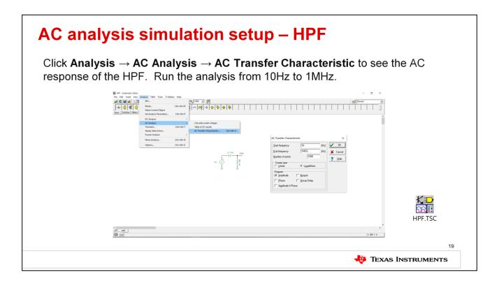
Let's again validate our analysis by running a TINA-TI simulation! Download the embedded TINA file and open it. Run an AC sim as before by clicking "Analysis," then "AC Analysis," and "AC Transfer Characteristic." The simulation settings box will pop up. Sweep the input signal from 10Hz to 1Mhz and hit "OK" to run the sim.
