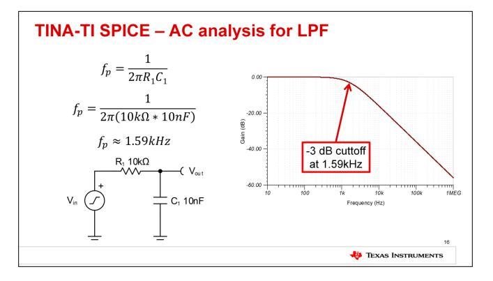
On the right we can see our simulation results. Indeed, the overall response of the circuit matches our expectations. There is a low frequency segment of 0dB of gain followed by a pole frequency and a region of -20dB/decade of gain. True to its name, the low pass filter passes signals of lower frequency and attenuates those at higher frequency. Using TINA's cursor function, we can place a cursor on the -3dB point to double check our calculation and indeed find that our pole comes in at 1.59kHz.
