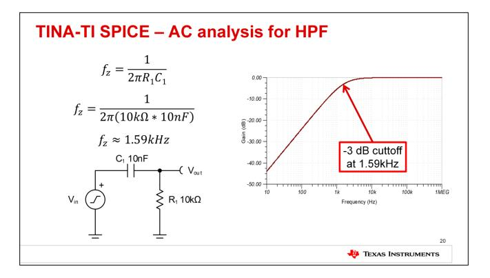
Again, the overall response of the circuit matches our expectation. The high pass filter attenuates signals at low frequencies and allows the higher frequency signals to pass. Using TINA's cursor function, we can place a cursor on the - 3dB point to double check our calculation and indeed find that our zero comes in at 1.59kHz.
