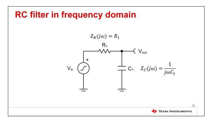
Having covered the time domain, let's move on to the frequency domain. Recall that a resistor has an impedance that is independent of frequency while a capacitor has an impedance that is inversely proportional to frequency. Analog engineers make use of these properties to design frequency filters with RC circuits.
