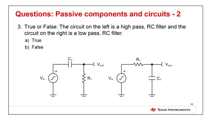
Question 3. True or False: The circuit on the left is a high pass, RC filter and the circuit on the right is a low pass, RC filter. The correct answer is true. Remember that for a high pass filter the current first passes through the capacitor and then the resistor while the opposite is true for the low pass filter.
