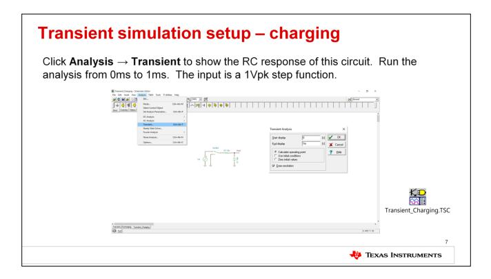
Let's first simulate a charging circuit. The TINA circuit is embedded in this presentation for your convenience. First, open the TINA circuit. Note, that the supply voltage is set to emulate a step function with an amplitude of 1V and a 100µs delay. Next, click "Analysis" and "Transient" to set up the simulation. We will run the sim for 1ms. Press "OK" to run the sim.
