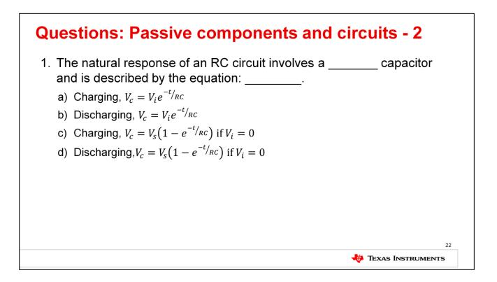
Question 1. Fill in the blank. The natural response of an RC circuit involves a \_\_\_\_\_ capacitor and is described by the equation: \_\_\_\_\_\_. The correct answer is "B." The "natural response" of an RC circuit refers to its ability to discharge and is described by the equation " $V_c = V_i$  times 'e' to the –t/RC."
