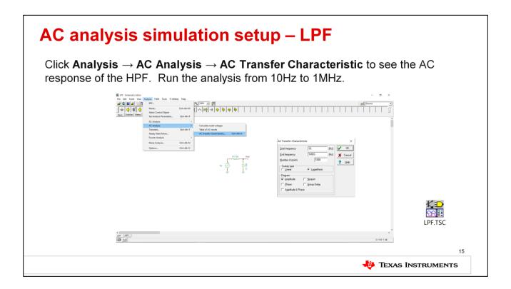
Let's now validate our analysis by running a TINA-TI simulation! The TINA file used is embedded in this presentation for your convenience. After opening the file, we can now run an AC sim. This can be done clicking "Analysis," then "AC Analysis," and finally "AC Transfer Characteristic." The simulation settings box will then pop up. We will sweep our input signal from 10Hz to 1Mhz. When you're ready, hit "OK" to run the sim.
