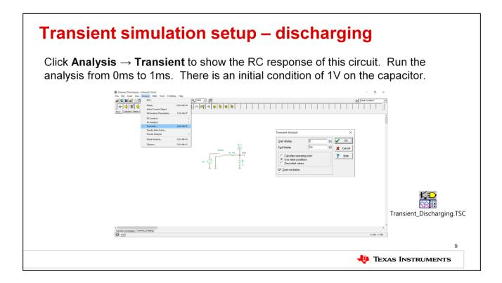
The transient response of a discharging RC circuit can be found in the same manner. This time, the voltage supply is disconnected and an initial condition of 1V is placed across the capacitor. The circuit is now tied to ground. The TINA file for the circuit used is embedded on this slide.
