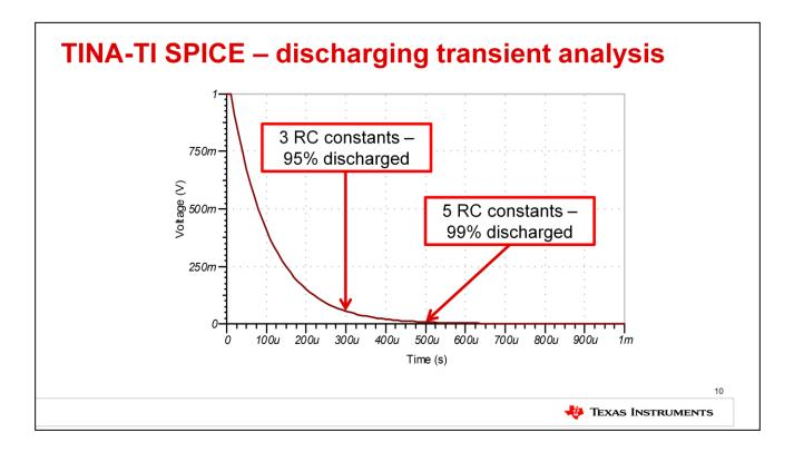
The natural response of the simulated RC circuit shows an exponential decay asymptotically approaching zero, as expected. After 3 time constants, or 300µs, 95% of the original charge is lost and the voltage level has fallen to 5% of the initial voltage level. In this case, that would be 50mV. Similarly, allowing 5 time constants, or 500µs, to pass will leave only 1% of the original voltage across the capacitor.
