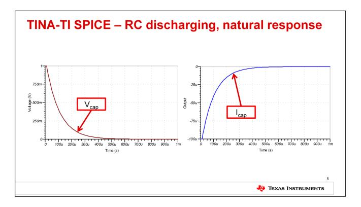
A similar SPICE analysis can be run for a discharging RC circuit. Here, an initial voltage of 1V is applied to the capacitor. Then at time 0, the RC circuit is suddenly switched to ground. The voltage across the capacitor decays exponentially, as expected, and the current through the capacitor corresponds to the change in voltage. Note that, in this case, the sign of the current direction is flipped because the current is set to flow in the opposite direction.
