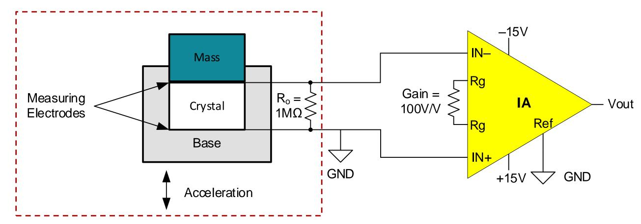
Assume IA input bias current =  $2.5 \mu A$  and the gain of the circuit is 100 V/V
