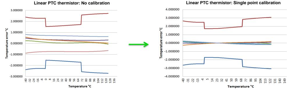
NTC: Multi-point calibration (requires temperature chamber) Linear PTC: Single point offset correction at room temp (no chamber)
