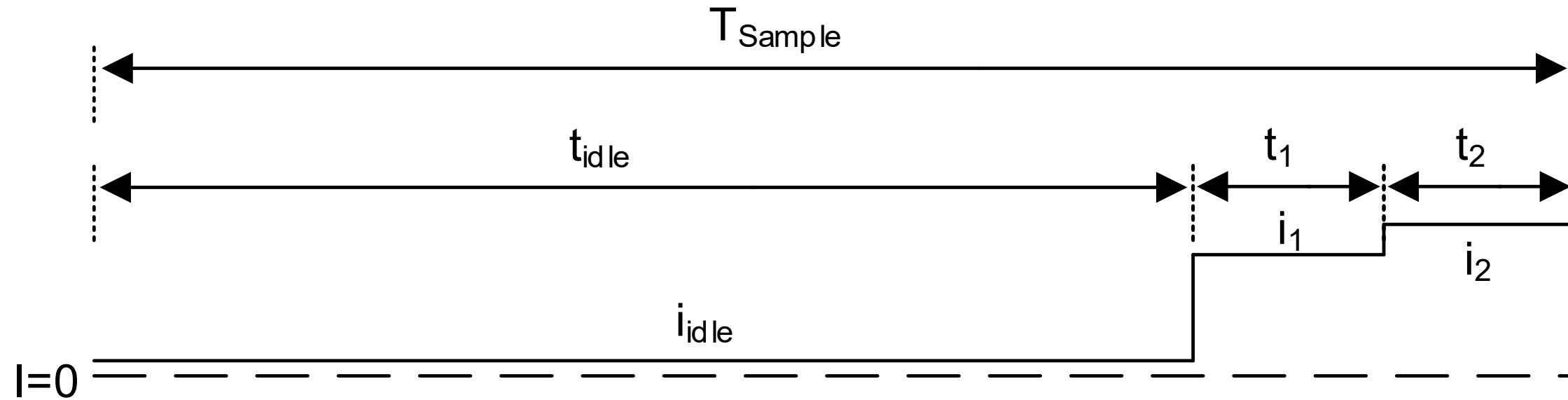
$$I_{AVG} = \frac{t_{idle} \times i_{idle} + t_1 \times i_1 + t_2 \times i_2}{T_{sample}} \quad t_{idle} = T_{sample} - (t_1 + t_2)$$
