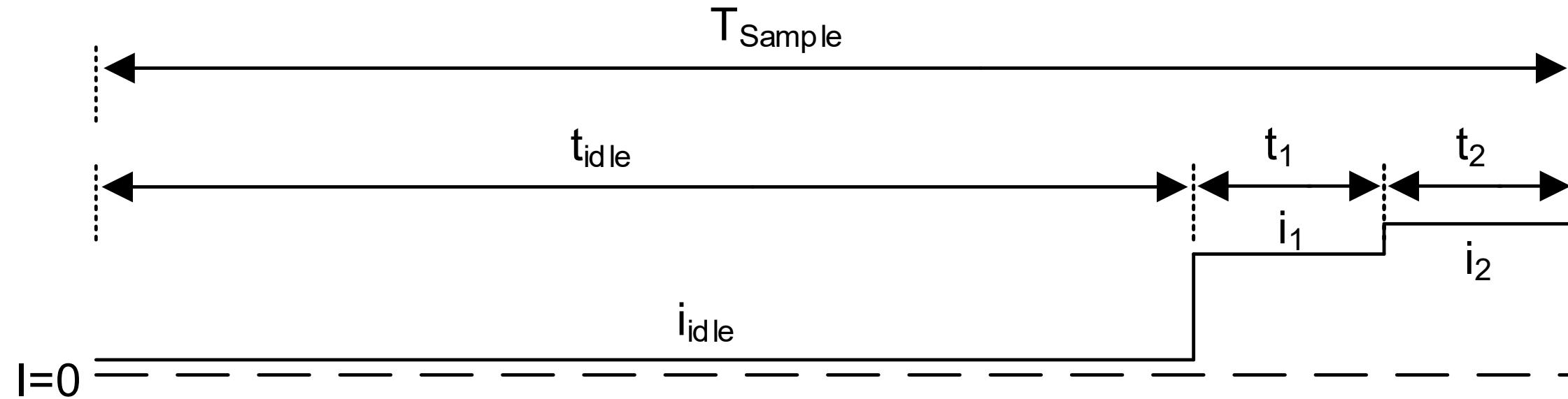
$$I_{AVG} = \frac{t_{\text{idle}} \times i_{\text{idle}} + t_1 \times i_1 + t_2 \times i_2}{T_{\text{sample}}} \quad t_{\text{idle}} = T_{\text{sample}} - (t_1 + t_2)$$
