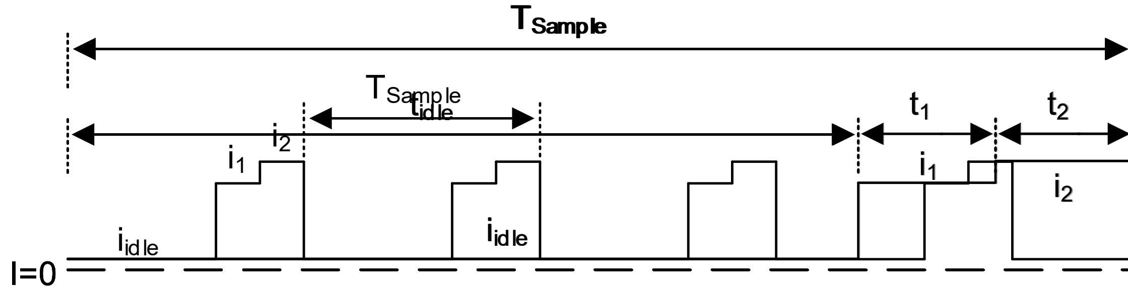
$$I_{AVG} = \frac{t_{idle} \times i_{idle} + t_1 \times i_1 + t_2 \times i_2}{T_{sample}}$$
