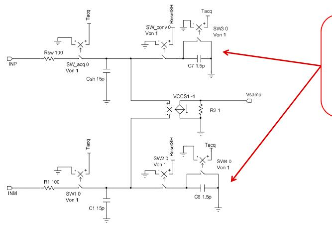
The reset capacitors deplete the charge on the sample and hold capacitor by 10% at end of conversion cycle. The old model reset to zero. Assuming the input signal is DC, the input capacitor looks like an effective capacitance of 1.5pF in this example.
