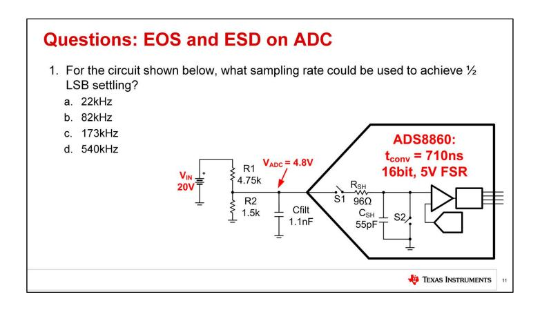
Question 1, For the circuit shown below, what sampling rate could be used to achieve ½ LSB settling?
