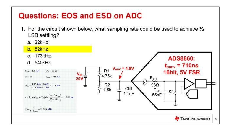
The correct answer is "b. 82kHz". The input impedance is the parallel combination of R1 and R2. This is used with the settling equation to find the acquisition period and finally the sampling rate.
