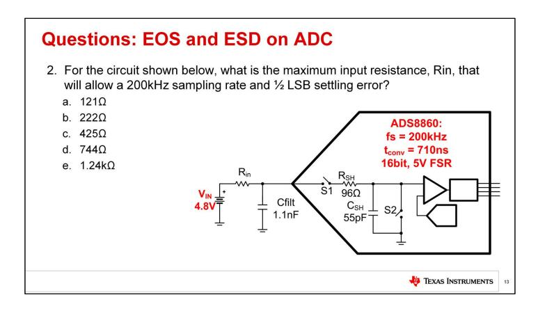
Question 2, For the circuit shown below, what is the maximum input resistance, Rin, that will allow a 200kHz sampling rate and ½ LSB settling error?
