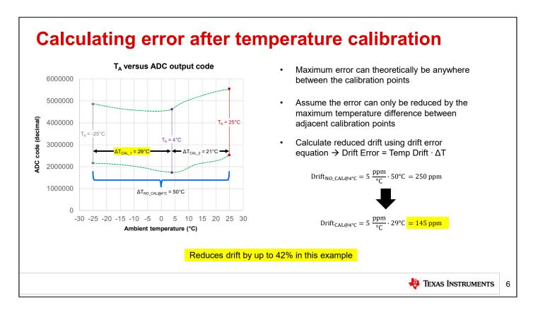
This plot was introduced on the previous slide, and shows how multiple calibration points can be required for systems with nonlinear behavior over temperature. Let's make some observations about the behavior of temperature error so we can estimate how much the calibration process reduces it
