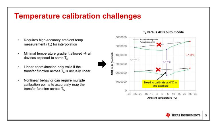
One important challenge with this temperature calibration process is that the ambient temperature must be known to be able to use the linearization equations introduced on the previous slide. This requires some method to accurately determine the system temperature, such as a discrete temperature sensor. This can increase the cost, power consumption, and complexity of the system
