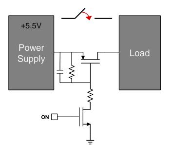
The two main functions a **load switch** can provide to a system is **power protection** and **power distribution**
