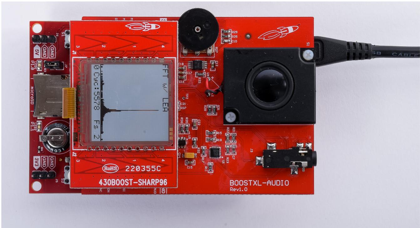
图 6. Stacked LaunchPad and BoosterPacks Reference Design
