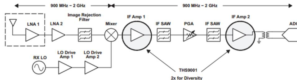
Figure 21. Example Single Conversion Receiver Architecture
