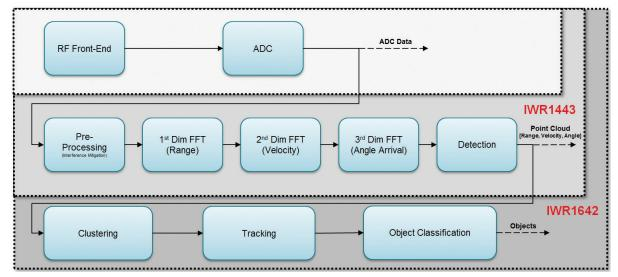
Figure 2. mmWave signal processing chain.
