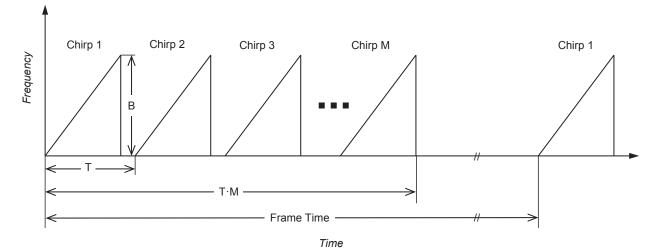
*Figure 4.* Frequency vs. time graph depicting a fast FMCW frame where B is the chirp bandwidth, T is the chirp repetition time (which could be a few tens of microseconds) and T·M is the total active chirping time in one frame. The frame time includes an idle time that may be a few tens of milliseconds.
