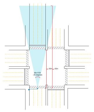
*Figure 5.* Example intersection with overhead radar sensor mount and azimuth field of view of 25 degrees covering a four-lane stop bar at a distance of approximately 30 m and an approach of approximately 60 m.
