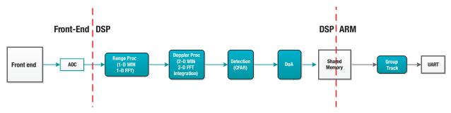
Figure 8. Processing chain flow for object detection, tracking and visualization for traffic-monitoring example.
