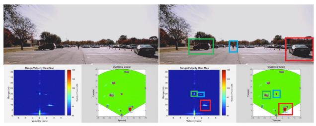
*Figure 3.* Range, velocity and angle information from mmWave sensors in an example parking lot scene. The graph with the blue background is a range/velocity heat map, where moving and nonmoving objects and their velocities are identifiable; the graph with the green background is a range/angle visualization. Colored boxes highlight the moving and nonmoving vehicles and pedestrians in the scene.
