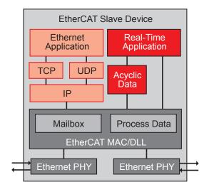
Figure 3. Components of an EtherCAT node.
