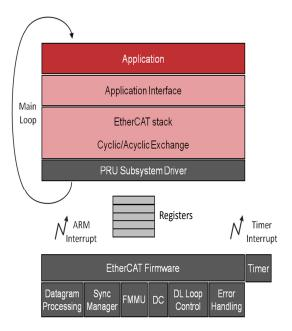
Figure 11. EtherCAT software integration.
