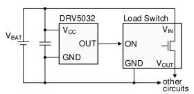
Figure 4. Typical Load Switch Schematic
