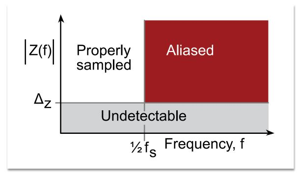
The **Nyquist Theorem** states that if the signal is sampled with a frequency of  $f_s$ , then the digital samples only contain frequency components from 0 to  $\frac{1}{2} f_s$ .
