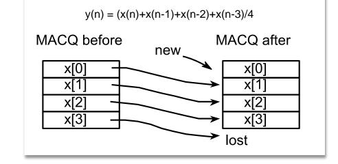
x[3] = x[2]; x[2] = x[1]; x[1] = x[0]; x[0] = ADC\_In6(); y = (x[0]+x[1]+x[2]+x[3])/4;
