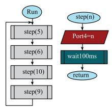
This motor spins clockwise when outputting the pattern 5,6,10,9 over and over. It spins counterclockwise when outputting the pattern in the other direction (5,9,10,6). The motor will stop if you leave its output at any of the valid patterns 5, 6, 10 or 9. Extend the FSM to have two inputs. If the input 0 or 1 the motor stops, if the input is 2 the motor spins clockwise, and if the input is 3 it spins counterclockwise.
