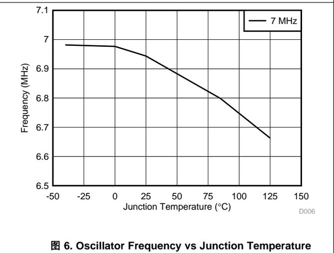
图 6. Oscillator Frequency vs Junction Temperature
