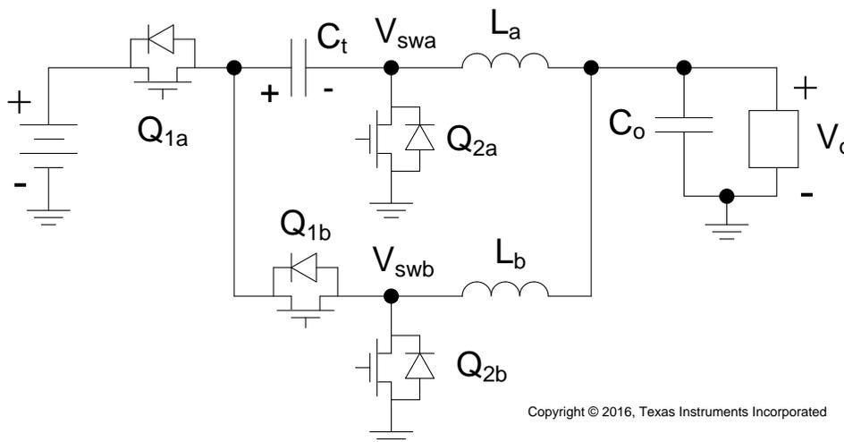
图 43. Two-Phase Series Capacitor Buck Converter Topology
