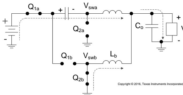
图 44. Phase A High Side MOSFET On
