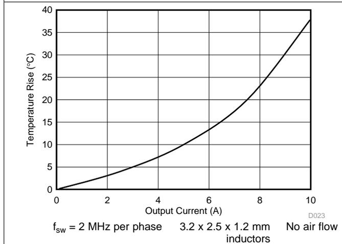
图 21. Case Temperature Rise vs Output Current
