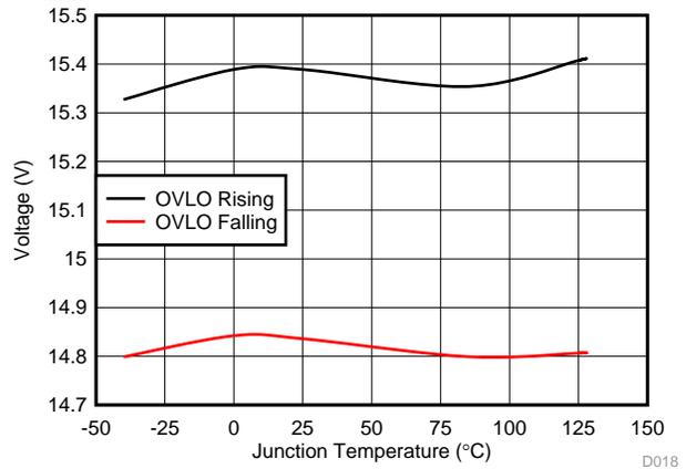
图 18. Overvoltage Lockout Threshold vs Junction Temperature
