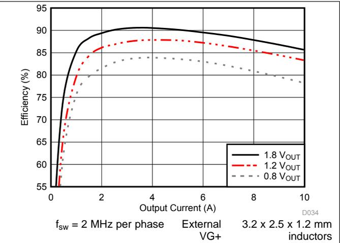
图 20. Efficiency vs Output Current for Output Voltage
