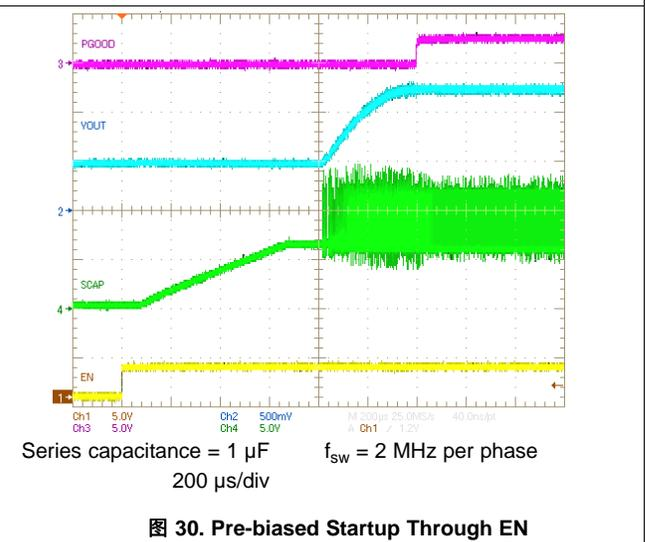
图 30. Pre-biased Startup Through EN
