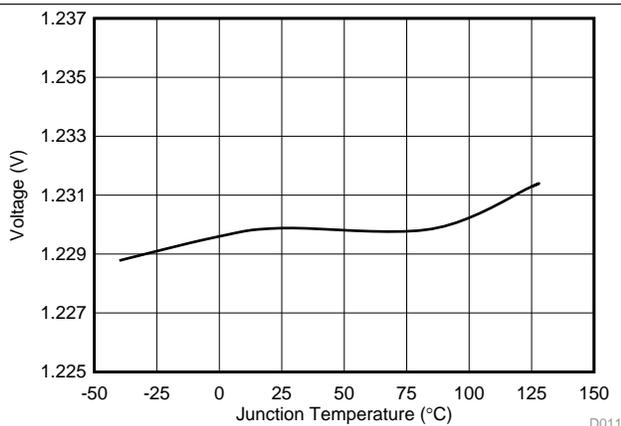
图 11. EN Pin Threshold vs Junction Temperature
