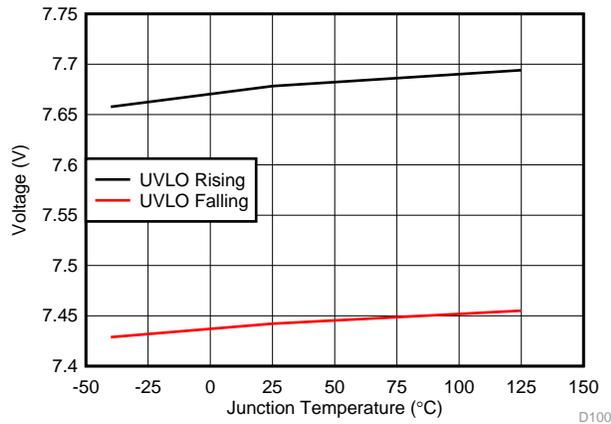
图 17. Undervoltage Lockout Threshold vs Junction Temperature
