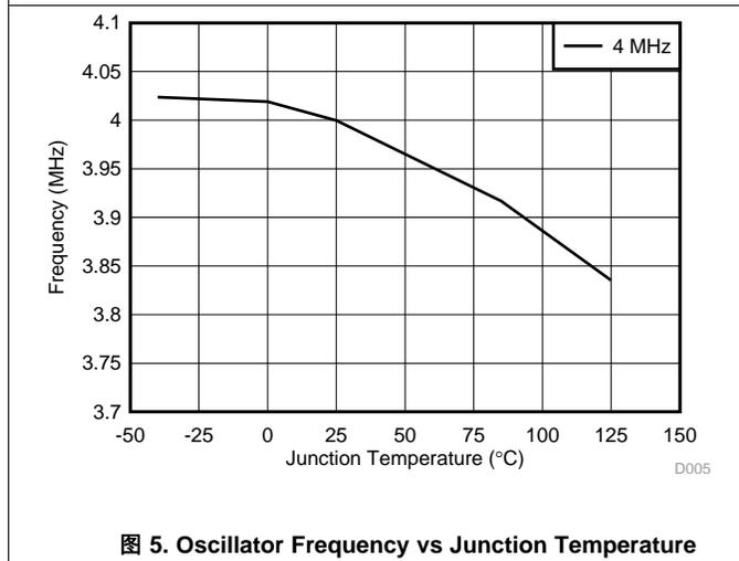
图 5. Oscillator Frequency vs Junction Temperature
