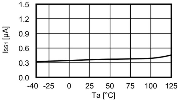
$V_{DET(S)} = 12.2\text{ V}$ ,  $V_{DD} = 13.5\text{ V}$ ,  $V_{SENSE} = 13.2\text{ V}$
