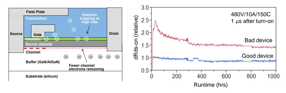
Reliability cell is able to monitor dRon evolution in GaN, and to detect bad devices
