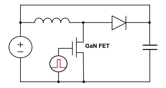
Double pulse mode: characterize switching dynamics Continuous pulse mode: Hard-switching stress
